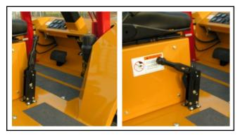
Engaged FIG. 23 Disengaged
